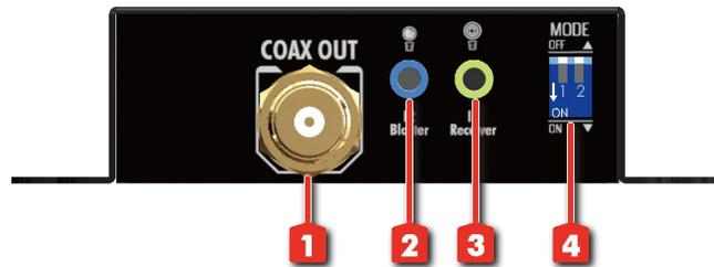
1. **COAX OUT:** Connects to a high standard coaxial cable here
